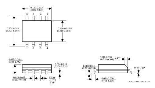
\*DIMENSION DOES NOT INCLUDE MOLD FLASH. MOLD FLASH SHALL NOT EXCEED  $0.006"\ (0.152\mathrm{mm})$  PER SIDE
