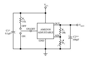
$$V_{OUT} = V_{REF} \times (R_1 + R_2)/R_1$$
